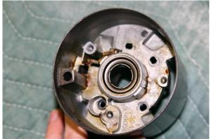
Zip Products 1-800-962-9632 has the Corvette Lock Housing Assembly still available with the bearing and plastic sector. The Zip part number is SC-447. Also Dr. Rebuild 1-800-866-9362 has the same assembly. The Doc's part number is 6521512
