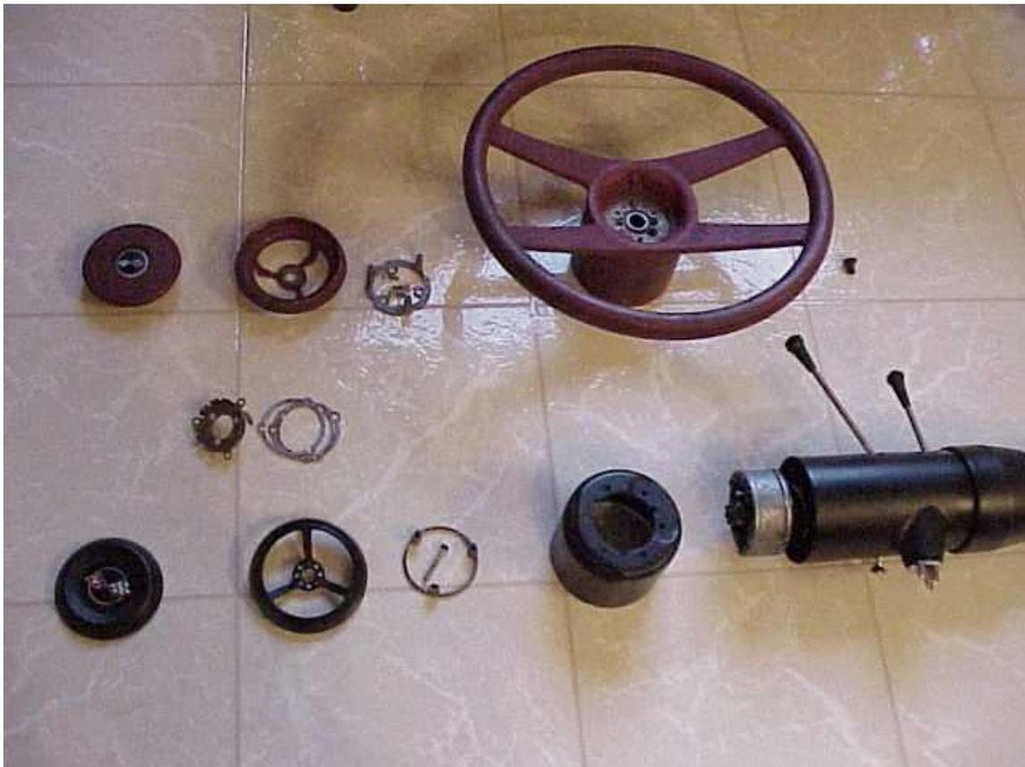
This picture is helpful in understanding the difference the differences even though not all of the parts are shown. The lower parts are the 1969-75 telescope lock and horn parts. The steering wheel is not shown. Note the aluminum colored hub on the steering column shaft.
