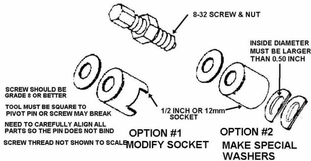
One other method to extract the pivot pins would be to thread a 8-32 screw into the end of each pin. Grip the screw with a slam puller tool. A few quick raps should draw the pin right out.
