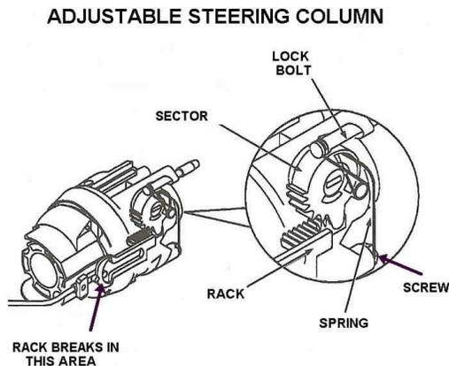
Install the bolt spring and spring retaining screw. Tighten screw to 35 inch lbs. Install the ignition switch actuator rod through the shroud from top and insert in the slot in the support
