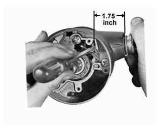
Don't be tempted to pry on the lock cylinder wings to get the lock cylinder moving. The wings will pop off and can't be put back on. The lock cylinder should slide right out.
