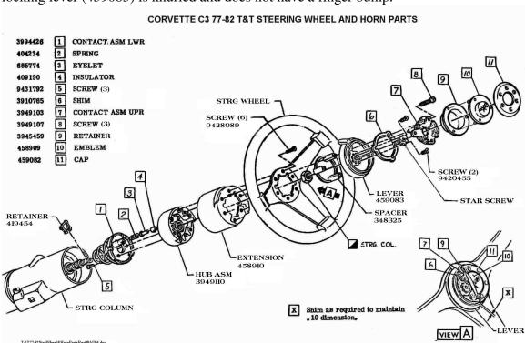
Use a screwdriver to pry up and lift the metal part (retainer #9) on the underside of the horn cap assembly from the horn contact. Do not pry directly on the cap itself.
