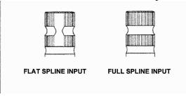
Early in the 1969 model year, steering gear input shafts and flexible coupling flanges were changed so that they had mating flats. The flat on the gear input shaft will be at 12 o'clock when the gear is exactly on center. You can see a portion of the input shaft flat sticking out from the flexible coupling flange in the photo on the previous page.
