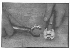
Separating Upper and Lower Shaft Sections
