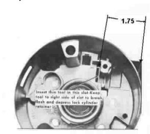
Fig. 1 Remove Lock Cylinder 1969 through Early 1979 Standard Columns
