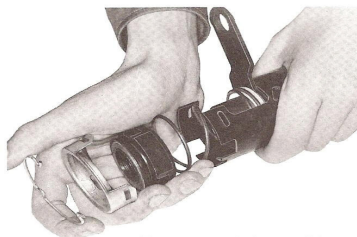
Remove retainer, slide lower bearing adapter out of steering column jacket.
