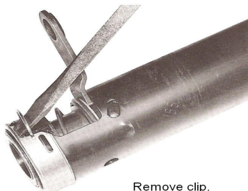
Remove clip. Lower lever on 1969-76 columns only.
