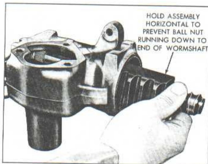
Fig. 3B-6--Removing the Wormshaft and Ball Nut--Typical
