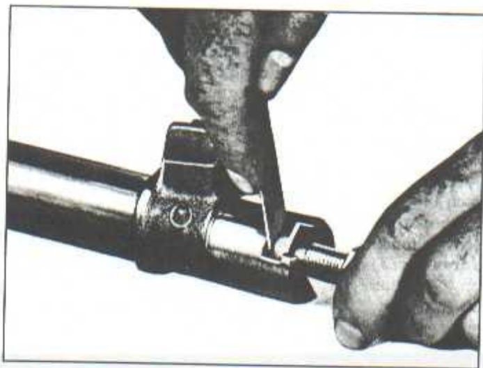
Fig. 3B-16—Checking Lash Adjuster End Clearance
