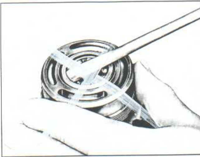
Fig. 3B-7—Removing Lower Bearing Retainer—Except Corvette
