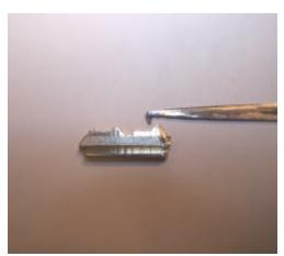
The following picture shows a course tooth hacksaw blade that has been modified to be used as a key bit extraction tool. Note that all of the teeth on the narrowed section of the blade have been removed except for the very last tooth right on the end. The end of a dental pick can be modified to act in the same way.
