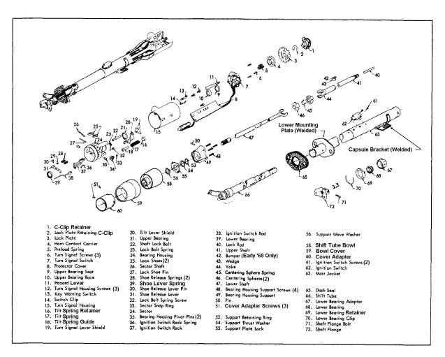
1969-76 CORVETTE TILT & TELESCOPING STEERING COLUMN BLOWUP
