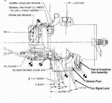
Sometime during the 1979 model year the dimmer pivot was changed to a steeper 46 degree angle. This brought the end of the turn signal lever close to the steering wheel rim without having a 30 degree bend.
