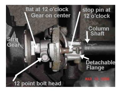
Picture of a typical GM steering gear, flexible coupling, and steering column flange looking over the front fender, straight down at the parts. Components are shown with the steering gear exactly on center. Many GM steering columns and intermediate steering shaft assemblies have a press fit, stamped lower flange instead of the cast, detachable type as shown.
