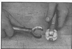
Separating Upper and Lower Shaft Sections
