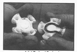
Joint Preload Spring in Centering Sphere
