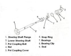
INTERMEDIATE STEERING SHAFT ASSEMBLY
