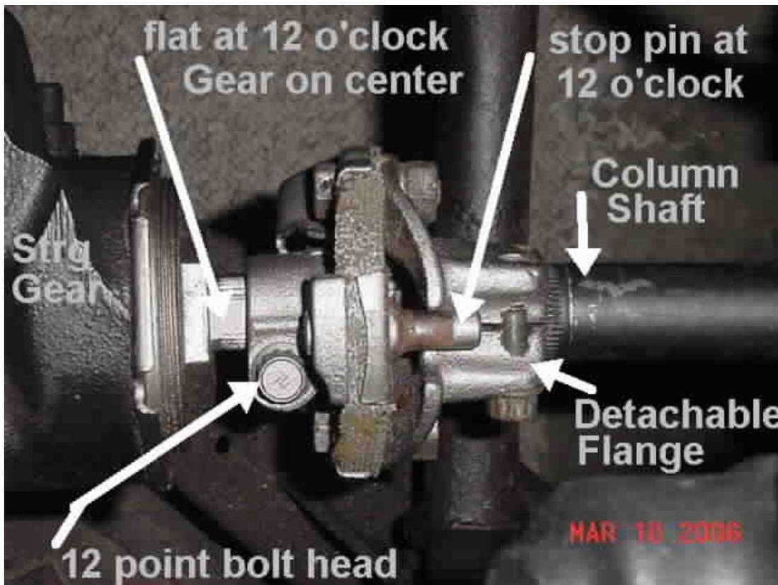
Picture of a C3 Corvette looking over the front fender, straight down at the steering gear, flexible coupling, and steering column flange. Components are shown with the steering gear exactly on center. Many GM steering columns have a press fit, stamped, lower flange instead of the cast detachable flange as shown.
