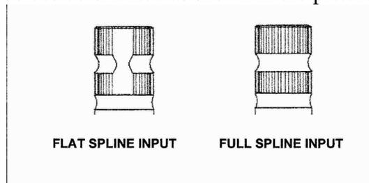
Early in the 1969 model year, steering gear input shafts and flexible coupling flanges were changed so that they had mating flats. The flat on the gear input shaft will be at 12 o'clock when the gear is exactly on center. You can see a portion of the input shaft flat sticking out from the flexible coupling flange in the photo on the previous page.
