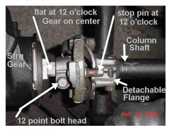
Picture of a C3 Corvette looking over the front fender, straight down at the steering gear, flexible coupling, and steering column flange. Components are shown with the steering gear exactly on center. Many GM steering columns have a press fit, stamped, lower flange instead of the cast detachable flange as shown.
