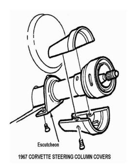
However, the curved plastic electrical connector is too large to pass through the gap. The shop manual says to just go under the dash and cut the wires. So if you are sure that your switch is toast (never to be used again) you can consider this approach. Otherwise, you will need to remove the wires from the connector and pull them through the escutcheon a few at a time.
