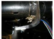
Make sure that you make note of the wire positions before you remove them from the connector. Straighten a heavy paper clip or use a very thin blade screwdriver; insert it into the connector from the contact side to disengage each wire and contact. Once you pop the wire and contact out of the connector, you should take a small knife blade and bend the tang back out so that it will engage the connector correctly upon reinstallation.
