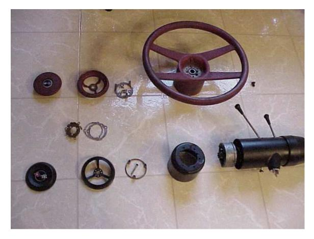
This picture is helpful in understanding the difference the differences even though not all of the parts are shown. The lower parts are the 1969-75 telescope lock and horn parts. The steering wheel is not shown. Note the aluminum colored hub on the steering column shaft.
